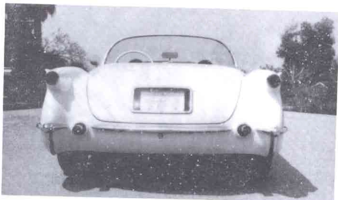
1954 rear view 53-54-55 the same, showing tail lights, bumper chrome (inner and outer), dual chrome exhaust extensions, recessed trunk license plate area, which has lights on each side to light up license plate at night. License plate is covered with curved plexiglass cover with a chromed outer boarder held in place with eight screws. Also some time in 1954 G.M. installed a small, approximately 2"x4" fiberglass box behind the license plate (visible with the trunk lid open) to house small gelucell bags in an attempt to keep the moisture at a minimum on the plexiglass license plate cover. This area in damp weather has a tendency to cloud up.
