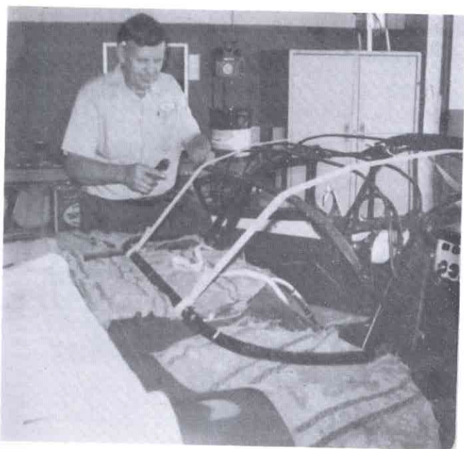
June 1974 — Rebuilding the soft top bows, framework and straps.
