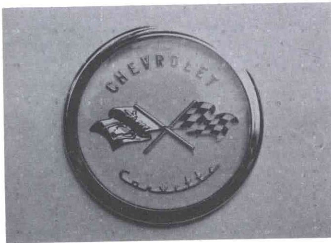
Original hub cap 1953-54-55. Tires 6.70x15, wide white wall tires mounted on sportsman red 15" rims. Sportsman red paint on perimeter slots and blue offsets Chevrolet emblem in hub cap centered.
