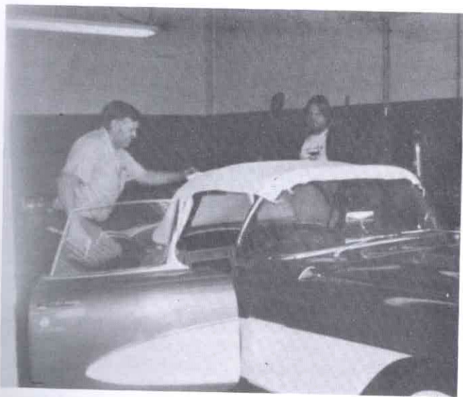
June 1974 — Mickey observes the fitting of the new top material to top frame.
