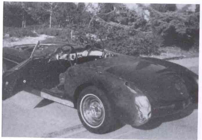
November 1972 — Windshield removed, and under door and left rear fender glass work completed.
