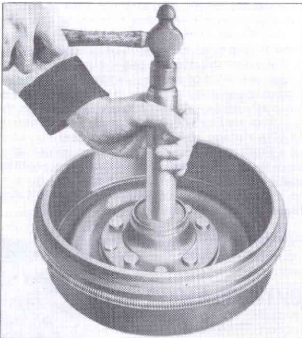
Fig. 6—Installing Bearing Cup
