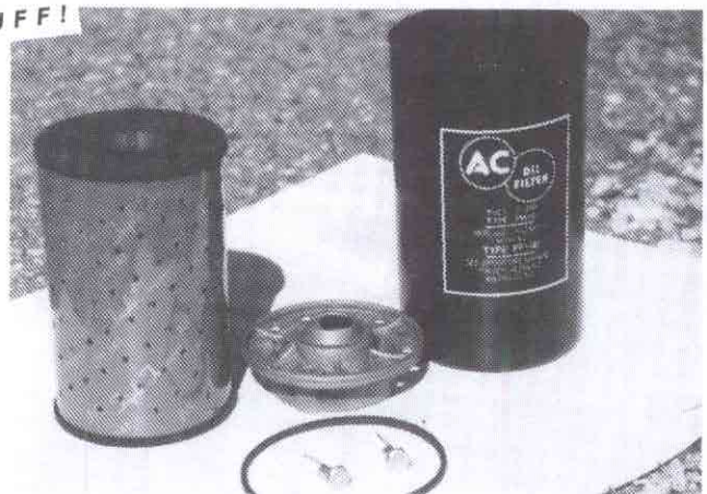
An original oil canister assembly new in box. Notice original filter blue AC.
