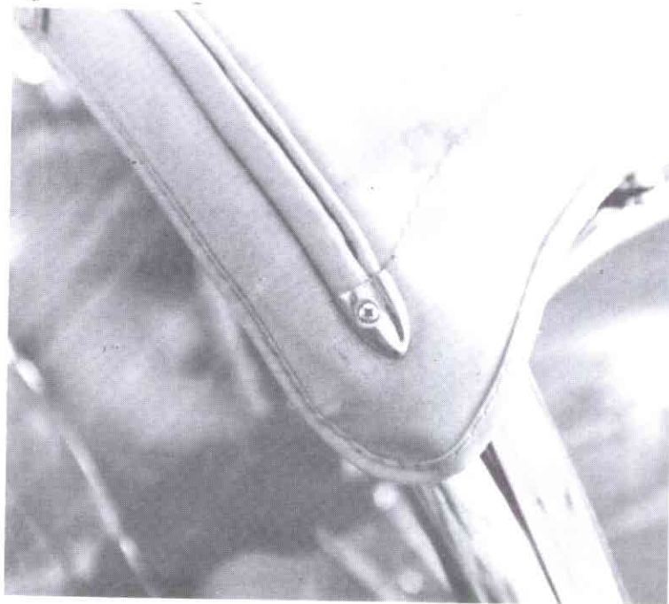
VIEW OF SOFT TOP RETAINER ORIGINAL DESIGN FOR '53 TO '62. THERE IS A LEFT AND RIGHT DIFFERENCE.
