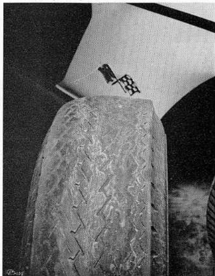
Fig. 6—Typical tire wear pattern.
